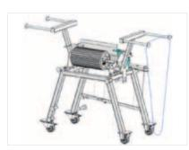
**Pic. 1 Cleaning cart:** With special fittings for comfortable cleaning of sanitizing-relevant machine parts, e.g. conveyer belts, pressure roller, knife holder etc.
